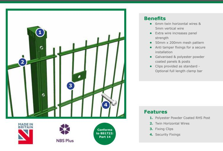
Zaun's Duo6 system is a twin wire fencing panel featuring two 6mm horizontal wires that sandwich 5mm vertical wires.
