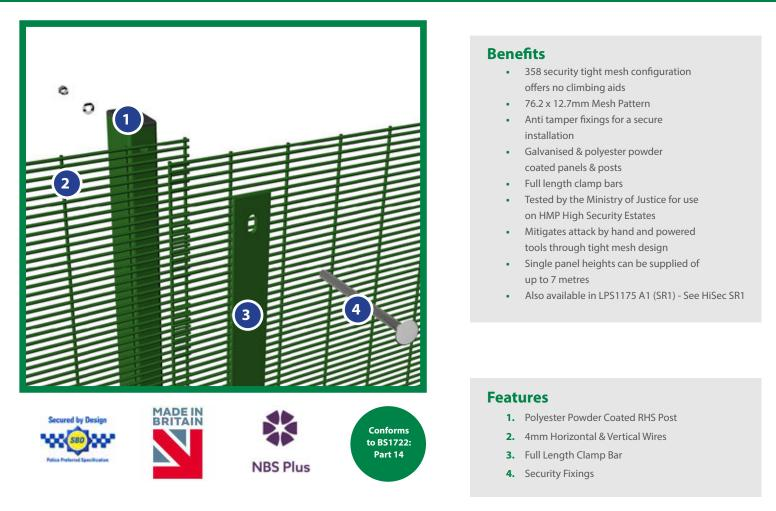
Zaun's HiSec 358 security fencing system uses the popular '358' welded mesh configuration. The close mesh (76.2 x 12.7mm) formation provides anticlimb properties that ensure that it is almost impossible to get fingers within the apertures to scale and climb the fence without the use of climbing aids. The attributes of the 358 mesh configuration make it an excellent solution for security applications.
